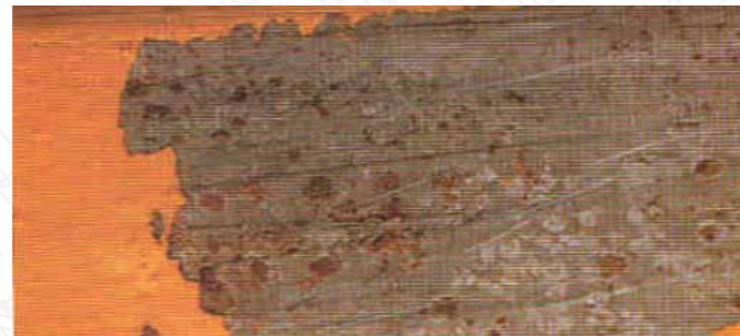
Image 3: Dotted under-rusting due to residual dross
