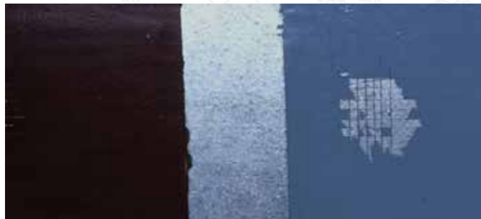
Image 1: Example of adhesion: left - special paint for the protection of galvanized sheet metal, right - "classic" universal paint for the protection of iron and wood
